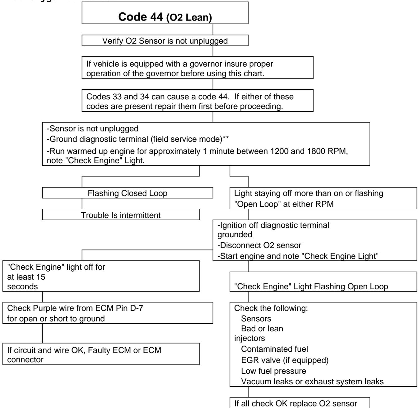
\*\* Service diagnostic mode is entered the same as Engine Off Self Test. Ground out Pin A and B on the ALDL connector with the engine running. Rapid flashing (approx 1/2 - 1 sec interval) is open loop. Flashing at a slower rate indicates closed loop.
